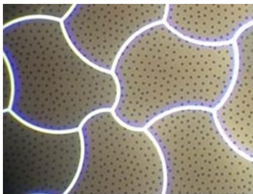
Figure 2. Microscopic Optical Image of Embossed Film
